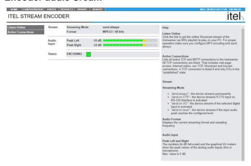
The audio streaming encoder module has the task of generating a streaming stream in the IP network, various encoding formats allow the transmission of the audio generated by the processor over the network to shoutcast / icecast servers, even in low latency, using RTP, UDP, Multicast or TCP / IP connectivity.
