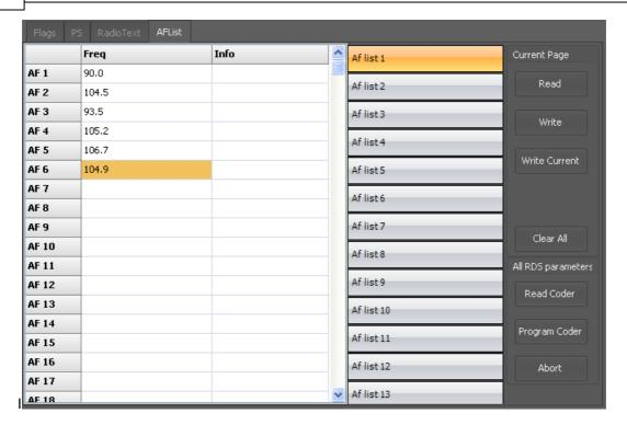
The main frequency (90.0MHz) is put in the first AF cell (AF1) and all alternatives are following from AF2 to AF6.
