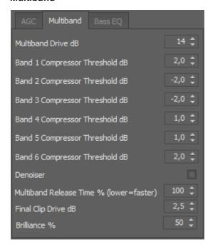
All six-bands limiters thresholds are adjustable in order to apply a dynamic equalization according to the user's taste. Lowering the limiting threshold of any band will result in attenuating the level of that band, while raising the threshold, will amplify its level.
