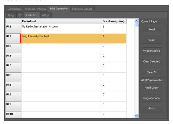
In this window, It is possible to enter the radiotext strings, each of which can be up to 64 characters long.
