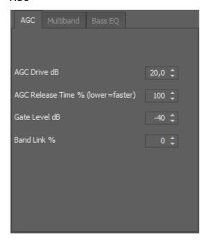
This window contains the settings for the dual band automatic gain control (AGC) block, placed at the head of audio processing chain.
