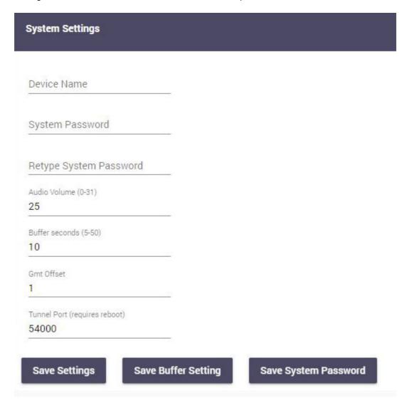
Device Name: device identifier. It is a character label available to the user to identify the device.
