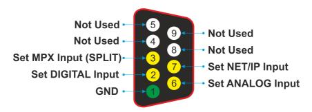
The inputs are activated by grounding the relative pin or by providing a voltage from 5 to 12VDC, in this case the jumpers placed on the board inside the device will have to be moved from the "CLOSE" to "VIN" position.
