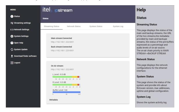
The module adds audio streaming decoding capabilities for receiving streaming MP3 / AAC + / HLS shoutcast servers or by using TCP / IP connectivity.
