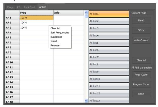
The frequencies must be inserted starting from the first list "Af list 1", cell AF1.
