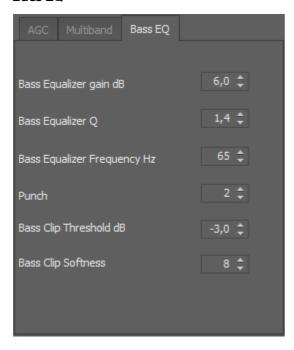
Bass Equalizer gain dB: gain (boost) of parametric equalizer.
