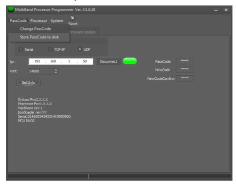
To protect the device from unauthorized operation, a security code can be set. The default code is 0000 (security disabled), but it can be changed through the following procedure:
