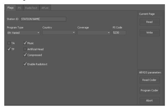
This window contains the configuration parameters of the RDS encoder.
